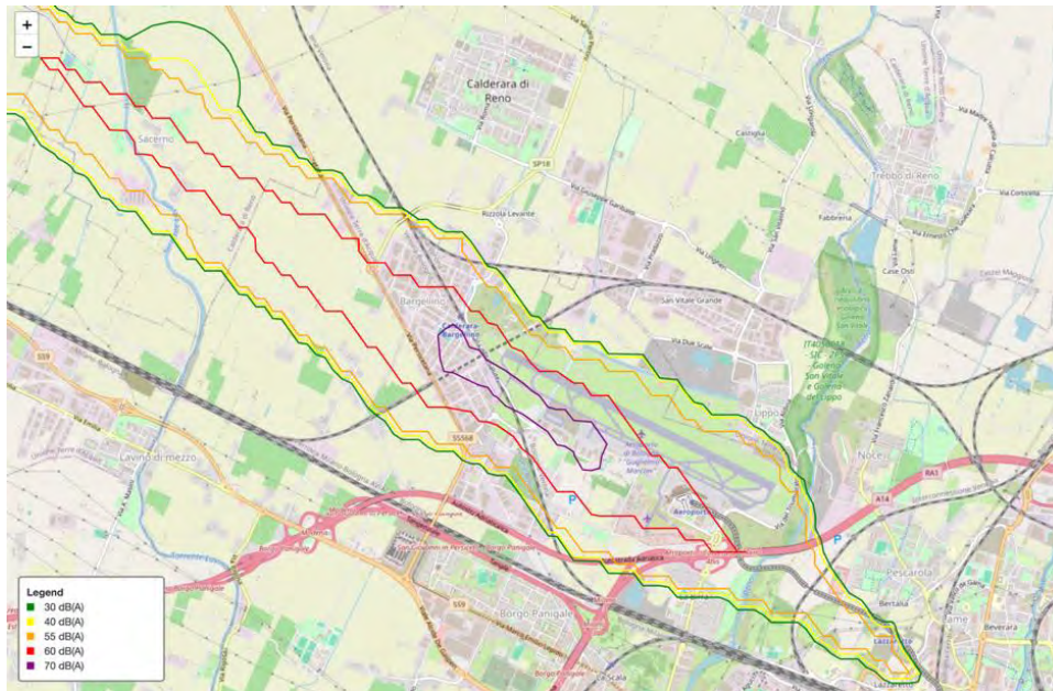
Figure 9 Overall L_{den} noise emissions L_{den(total)} , in dB(A), in Sacerno, northeast of Bologna Airport, considering existing noise sources from the Bologna airport, as well as those from the hypothetical wind turbine. Background map: OpenStreetMap.
