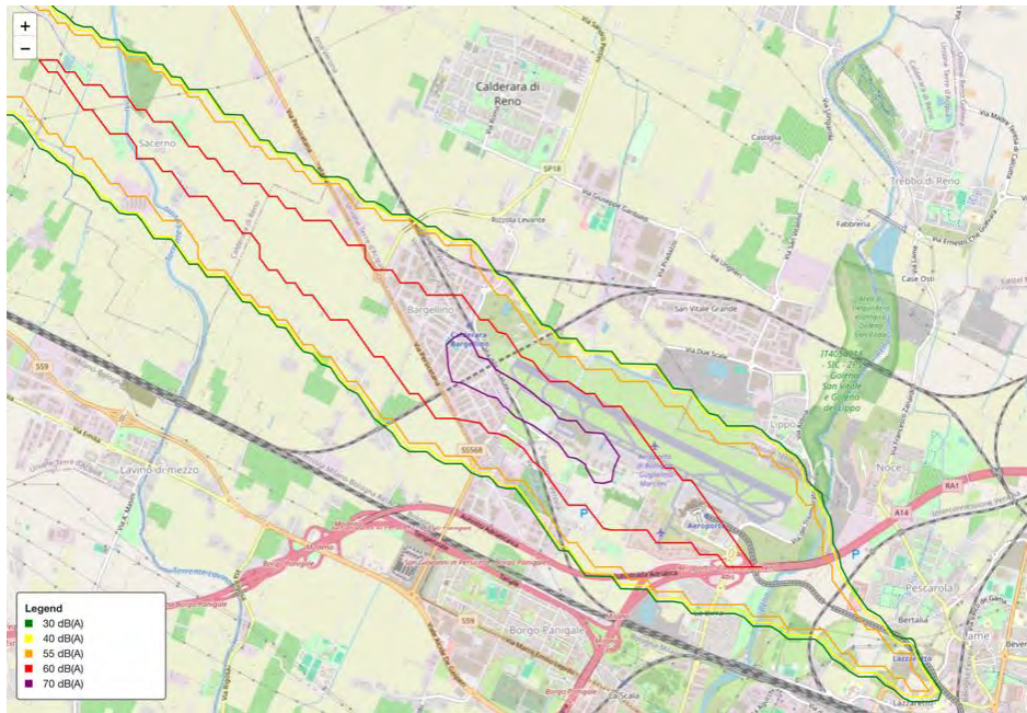
Figure 8 Existing L_{den} noise emissions L_{den(amb)} , in dB(A), in Sacerno, northeast of Bologna Airport, identified using European Noise maps data. Background map: OpenStreetMap.
