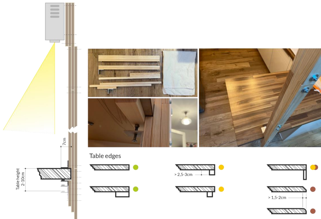
Figure 5 - Wooden construction for projector and camera mount and a classification of different table edges for their suitability
